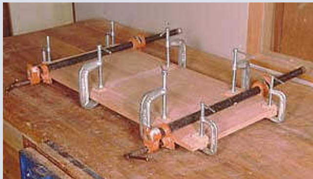
Photo 7- Gluing up the door. Wet out the parts, put on the bar clamps, then the C-clamps, then remove the bar clamps. Before you put on the C-clamps, be sure the door is flat.
