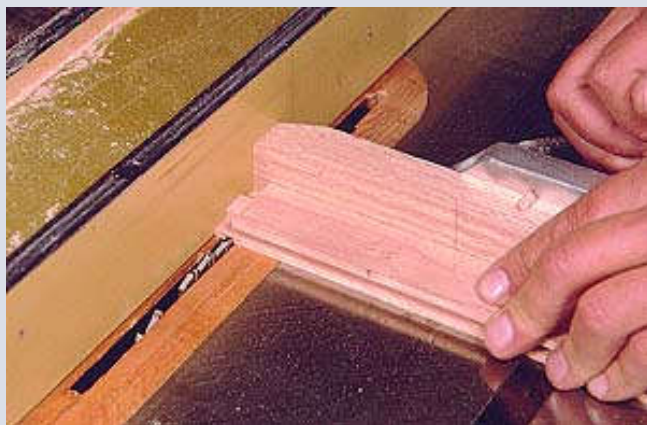
Sure Lock Miter Gauge With fence and flip stop.
