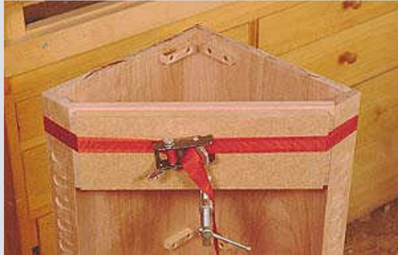
Photo 17- A band clamp (also called strap or web clamp) is the ideal tool for clamping odd shapes like this. The C-clamp just held the spacer in place while the band clamp was installed. An alternative to a
