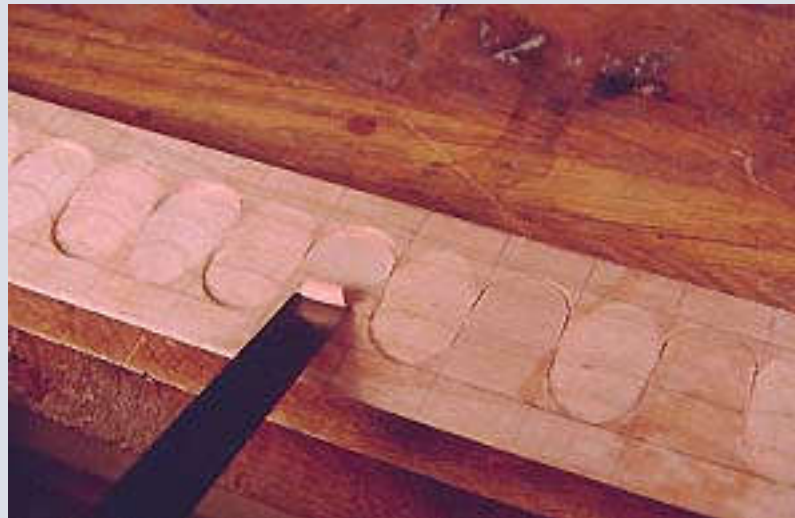
Photo 10- Make a sloping cut down into each of the half circles as shown.
