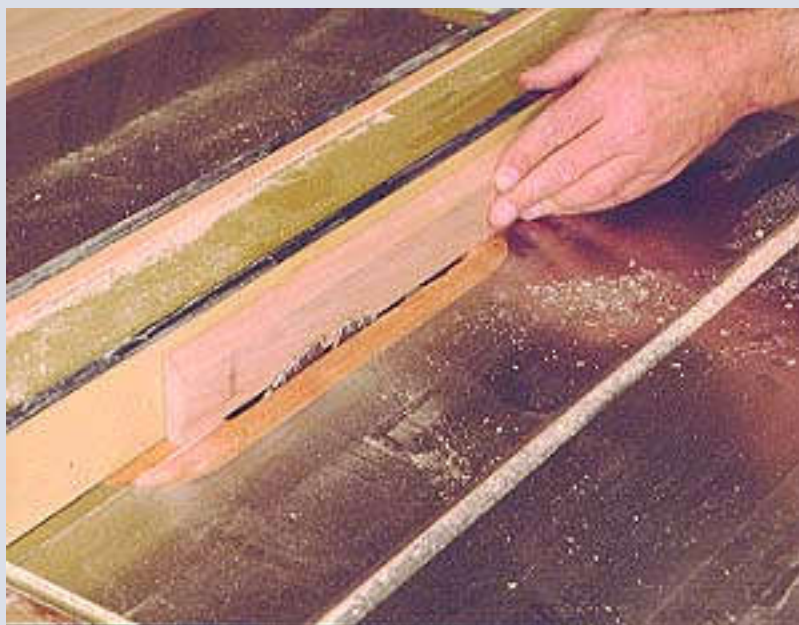
Photo 13- Make a shallow reference groove where the carcass parts join so that when you put it together the parts have a shoulder to sit against, keeping them in alignment.
