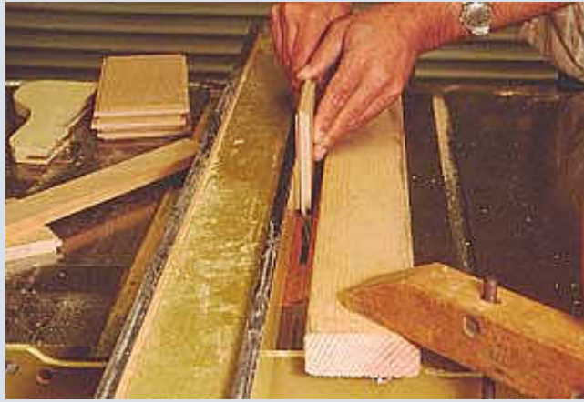
Photo 6- Cutting the panel tongues on the panels. The height of the cutter is going to determine the exact fit of the panels in the door frame parts. Test fit them while you have the setup going so you can make adjustments if necessary. Leave some room along the panel width for moisture related expansion.
