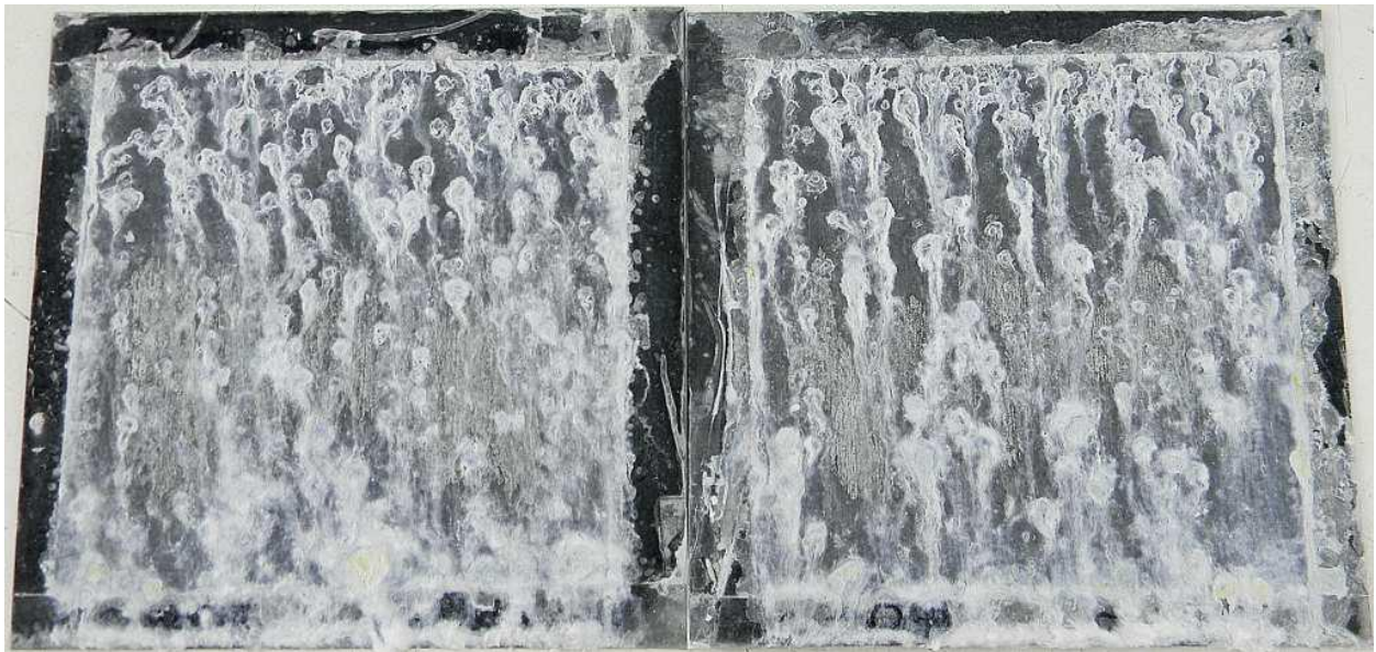
220332031 .0140" G90 Acrylic – 1008 hrs Salt Spray – ASTM B117
