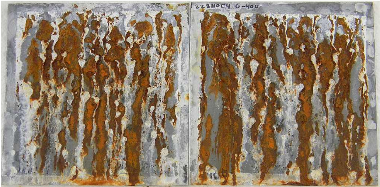
22311054 .0117" G40U - 1008 hrs Salt Spray – ASTM B117
