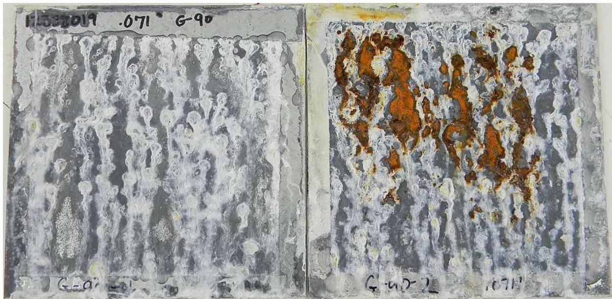
12338019 .071" G90 – 1008 hrs Salt Spray – ASTM B117
