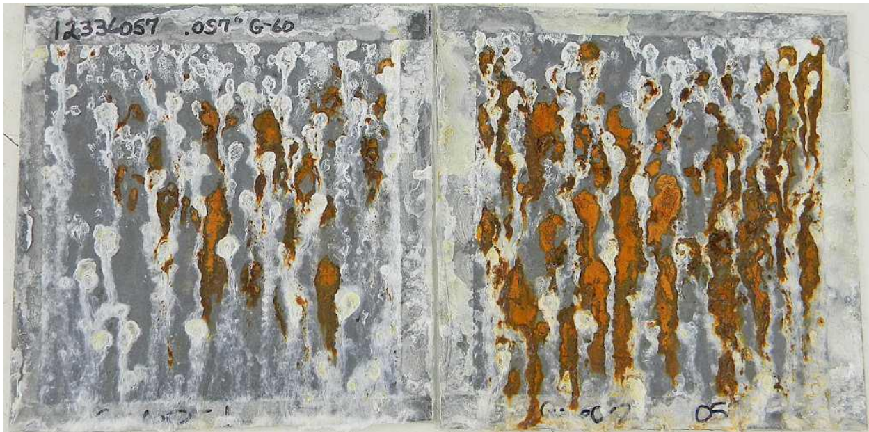
12336057 .057" G60 – 1008 hrs Salt Spray – ASTM B117
