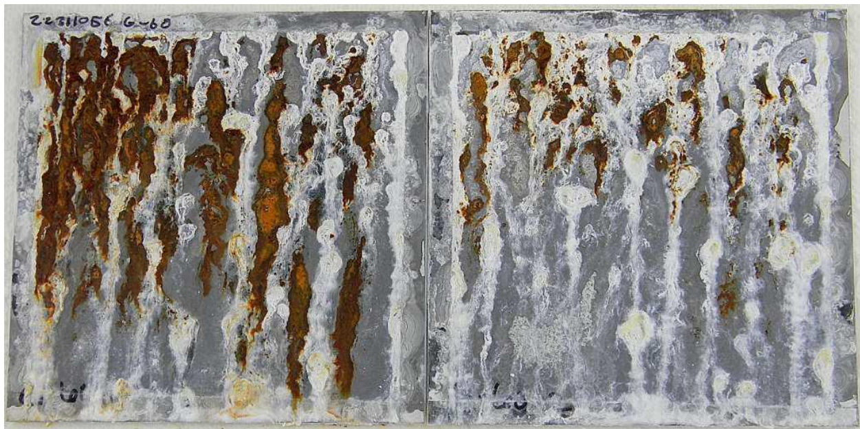
22311056 .0142" G60 - 1008 hrs Salt Spray – ASTM B117
