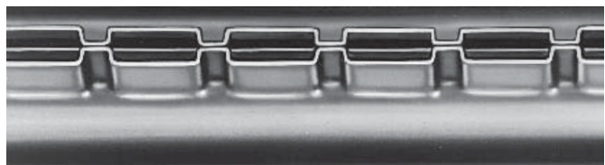
Figure 4.1 Burner Port Closeup
