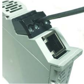
Figure 3 - Terminal Block Removal
