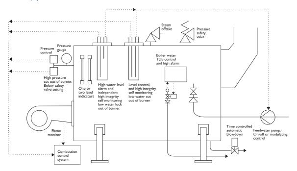
New installations should be manufactured to BS EN 12953, which requires additional limiters to be fitted.
