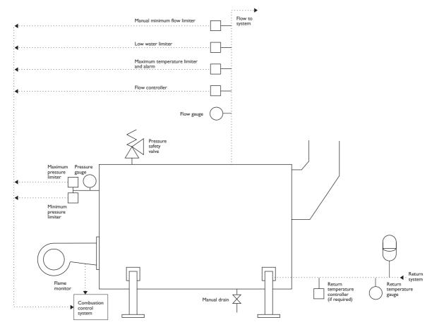
**Note:** For detailed requirements to suit different boiler types (eg steam cushioned) refer to BS EN 12953 Part 6 and SAFed PSG3 – Guidelines for the Operation of Hot Water Boilers. Solid fuels may require additional emergency cooling systems.
