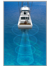
With a fairing, the beam is aimed straight down.
