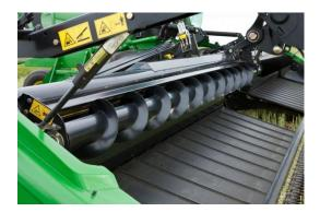
The cross auger helps deliver very bulky crops across the header onto the windrow. May also need case drain kit BE32510.
