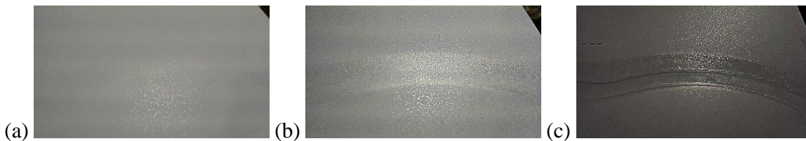
Figure 38. The three levels shown in a seal: (a) Level 0, (b) Level 1, and (c) Level 2.
