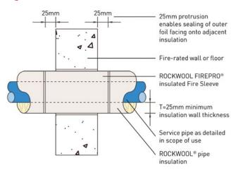
All joints to be taped with self-adhesive foil tape, including the joints where the insulated fire sleeve butts to existing insulation. To maintain the fire rating stated above, the minimum allowable length of sleeve is 50 mm. Insulated Fire Sleeves can accommodate irregularities in the division opening and the pipe O.D.up to 15 mm. Multiple pipe penetrations can be accommodated in conjunction with intumescent coated batts.
