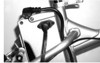
Electric Bikes with Seat Tube Mounted Battery (STB) Packs - Remove the power cable from the charger port and attach charger.
