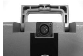
Electric Bikes with Rack Mounted Battery (RMB) Packs - Lift the battery pack handle to expose the charger port and attach charger.
