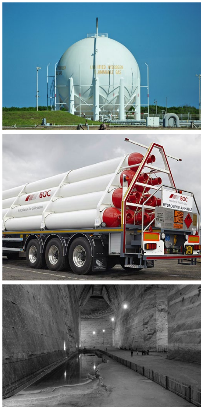
Figure 5: Hydrogen storage and distribution options; liquefied hydrogen tanks (top), tube trailers (middle) and salt caverns (bottom) 39
