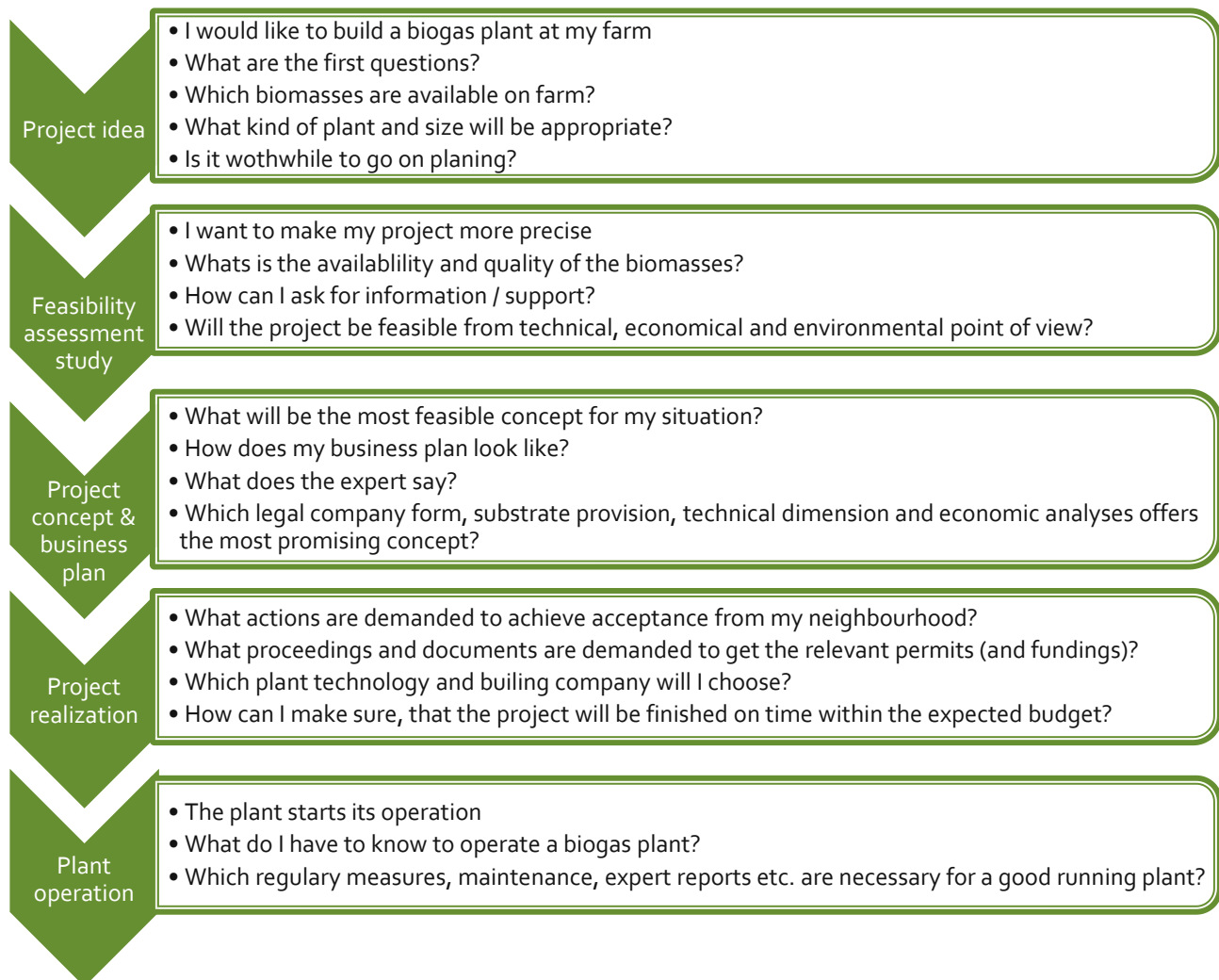
Figure 3: Essential project development phases and central questions for implementing a biogas plant [CASTILLO ET AL 2012, modified]
