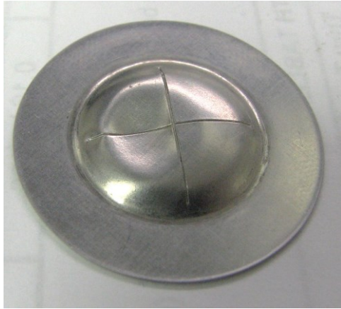
Figure 47 - Dent Caused by Water Freezing in Discharge Line
