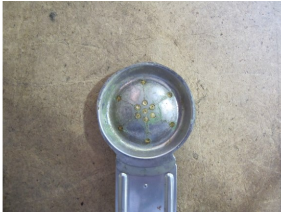
Figure 46 - Disk Subjected to Corrosion
