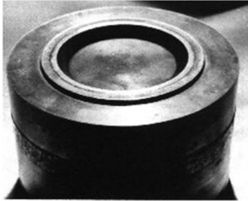
Figure 28 - Seating Surface of Disc deformed by Chattering
