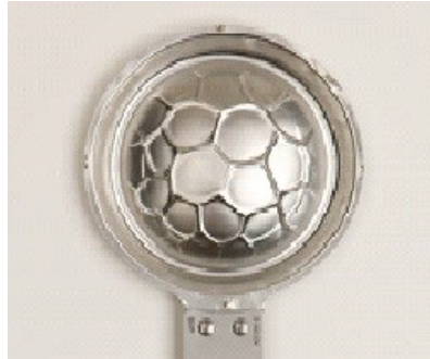
Figure 44 - Operating Ratio Exceeded then Subjected to Vacuum
