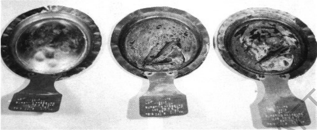
Figure 26 – Alloy 400 Rupture Disks Corroded in Sour Gas Service
