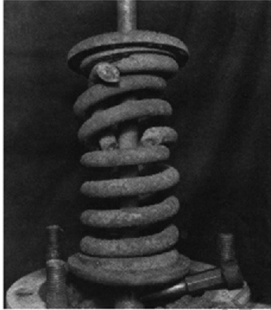
Figure 30 - Spring Failure Due to Corrosion
