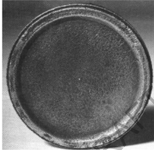
Figure 24 - Chloride Attack on 18Cr-8Ni Steel Disc
