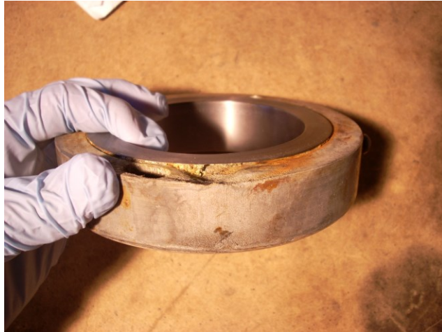
Figure 50 - Rupture Disk Holder Corrosion due to Leakage
