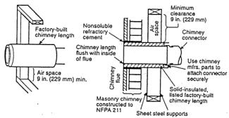
B Solid-insulated, listed factory-built chimney length of the same inside diameter as the chimney connector and having 1-in. or more of insulation with a minimum 9-in. air space between the outer wall of the chimney length and combustibles.
