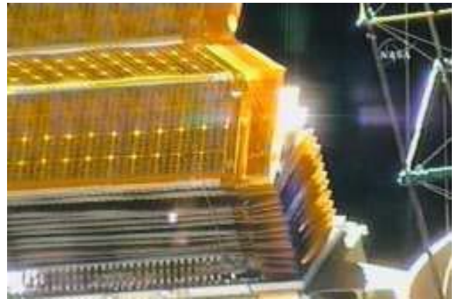
Figure 37. Stowed Solar Panel Being Unfolded for Deployment
