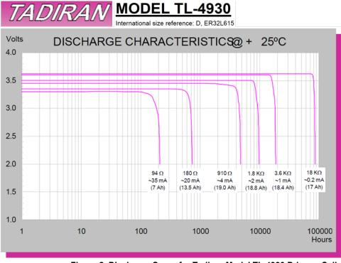
Figure 2. Discharge Curve for Tadiran Model TL-4930 Primary Cell Source: The Tadiran Company
