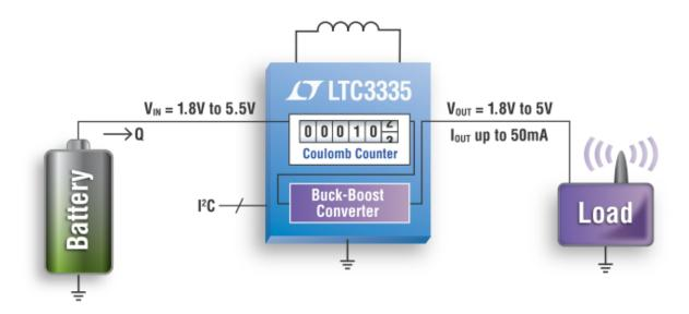
Figure 3. LTC3335 Buck-Boost Converter with Integrated Coulomb Counter
