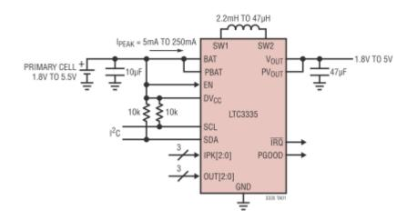
Figure 4. Simplified LTC3335 Application Schematic
