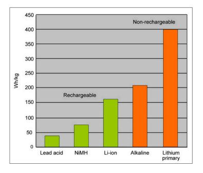
Figure 1. Energy Density of Rechargeable vs. Primary Cell Batteries Source: Battery University
