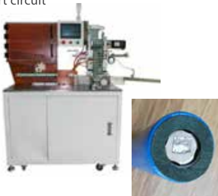
Fig. 13 – Insulator pasting machine
