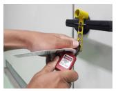
employee secures each energy-isolating device – typically with a lock as shown below. An authorized employee is one who locks out or tags out the energyisolating device and services the equipment.
