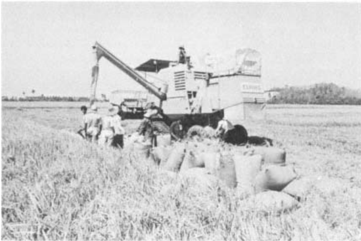
6. The combine-harvester. Workers are sewing shut the gunny sacks filled with harvested paddy.
