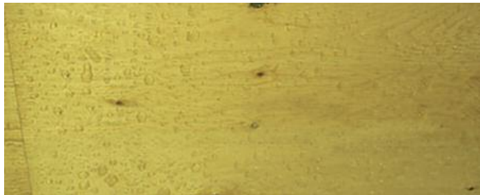
Photo shows example of the beading that occurs because of our coating process.
