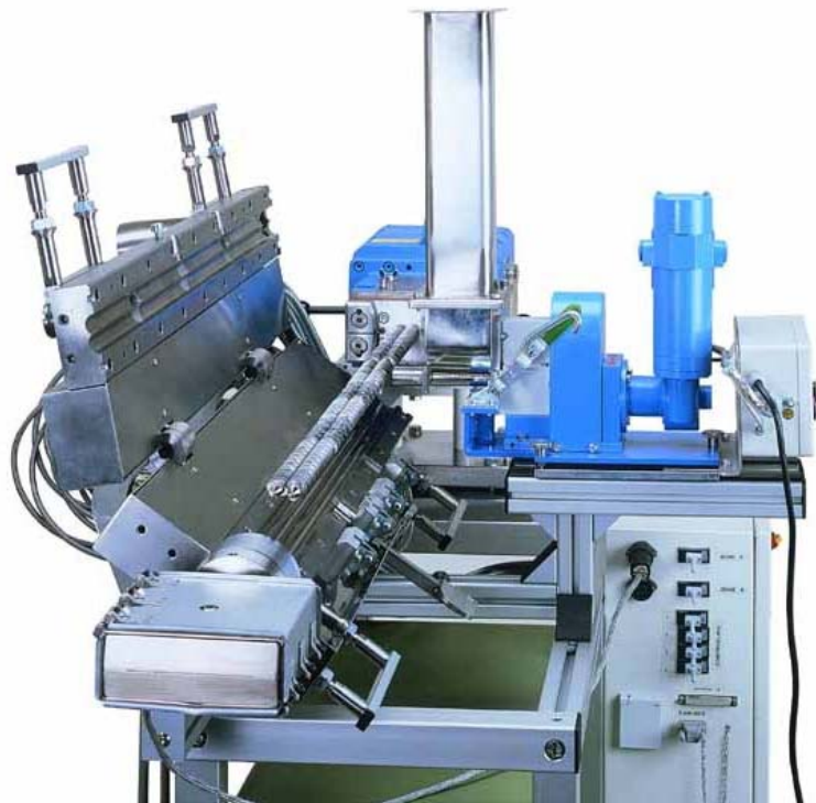
Figure 1-5-1: Extruder with horizontally divided barrel. Source: www.brabender.com
