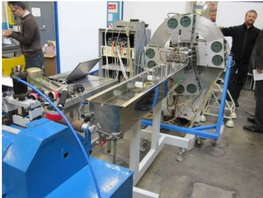
Figure 7-2-4: The downstream equipment (water bath and pelletizer)
