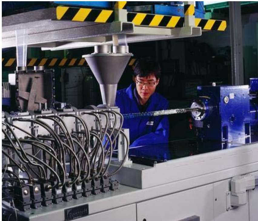
Figure 1-5-2: Extruder with extractable screw. Source: www.berstorff.de
