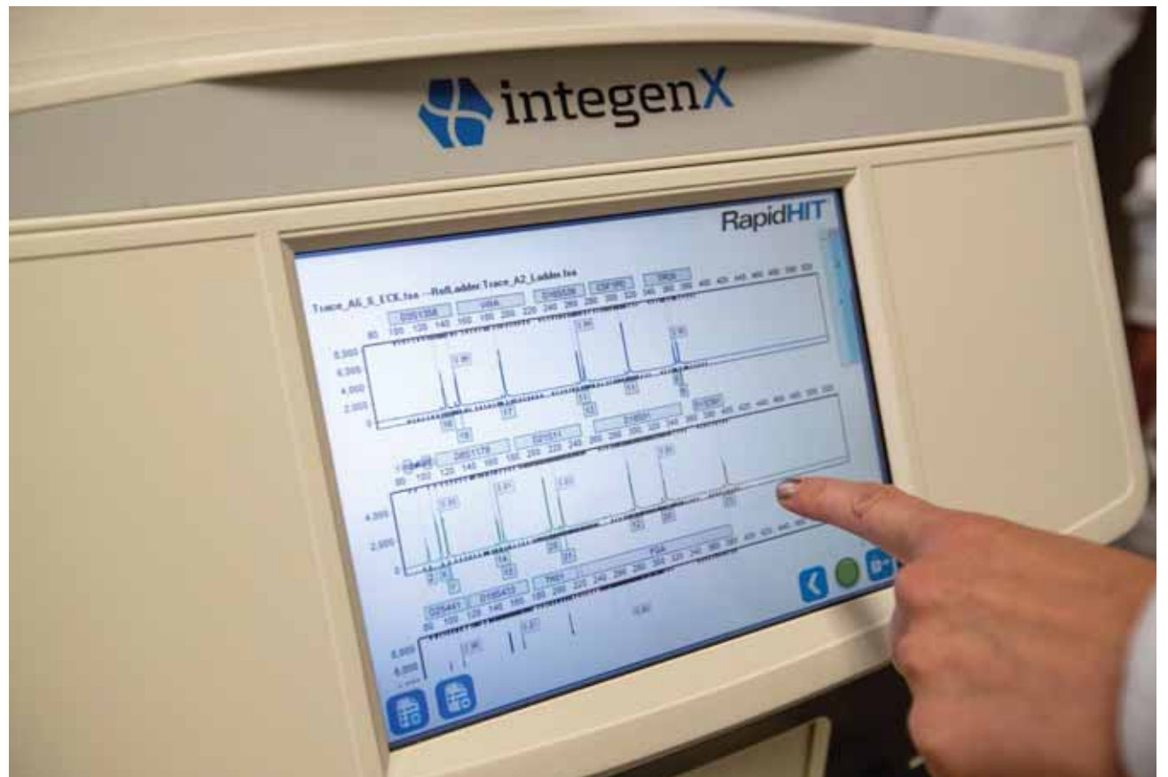
THE DEVICE: A DNA readout on a Thermo Fisher RapidHIT 200 Rapid DNA machine in Santa Ana.
