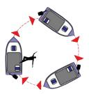
Every year, serious injuries and deaths occur when operators let go of the steering wheel or outboard steering handle while the boat is moving. The steering torque forces the motor to slam left
