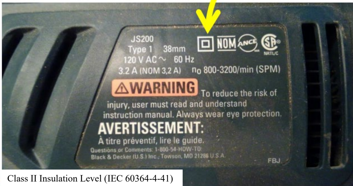
Symbol for "Double Insulated" tool (square inside a square)
