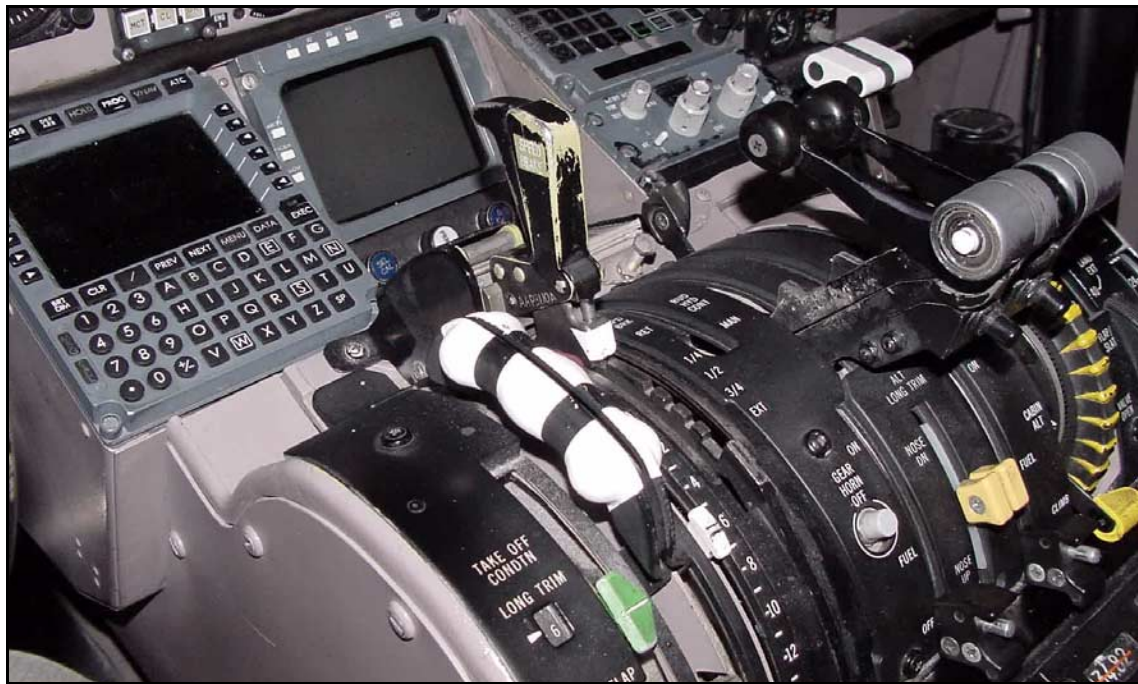
Figure 4. Spoiler Handle in the Unarmed Position
