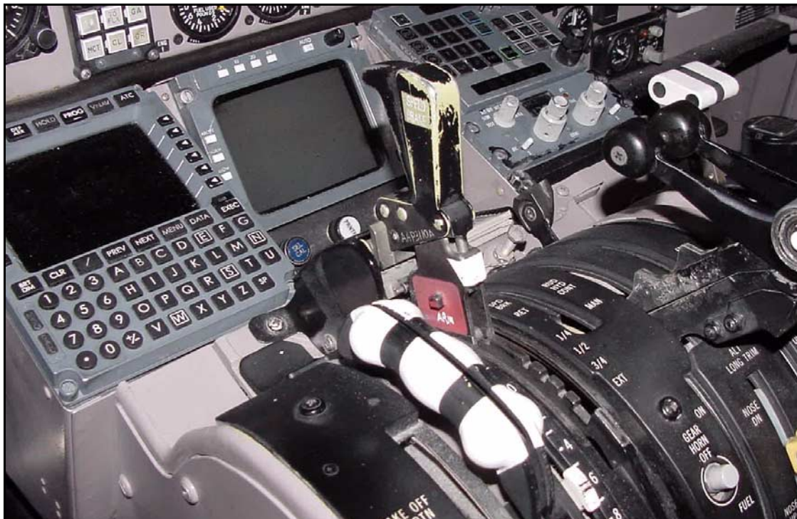
Figure 5. Spoiler Handle in the Armed Position
