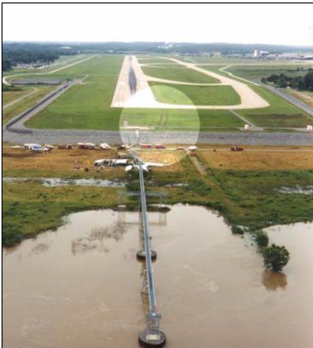
Figure 12. Aerial Photograph of Runway 4R/22L, Airplane Wreckage, and Runway 22L Approach Lighting System
