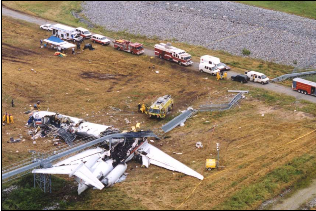
Figure 13. Airplane Wreckage and Runway 22L Approach Lighting System
