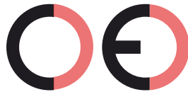
False CE Mark (too far)
