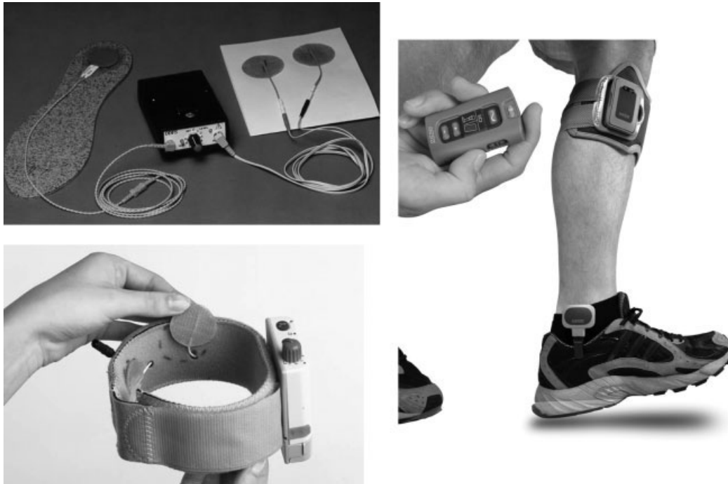
FIGURE 6. Three FDA-approved transcutaneous peroneal nerve stimulators. The Odstock Dropped Foot Stimulator (top left, courtesy of Department of Medical Physics and Biomedical Engineering, Salisbury District Hospital, Salisbury, UK.) and the wireless NESS L300 (right, courtesy of Bioness Inc., Santa Clarita, CA) both use a heel switch to trigger ankle dorsiflexion. The WalkAide (Bottom left, courtesy of Hanger Orthopedic Group/Innovative Neurotronics, Bethesda, MD) uses a tilt sensor to trigger ankle dorsiflexion.
