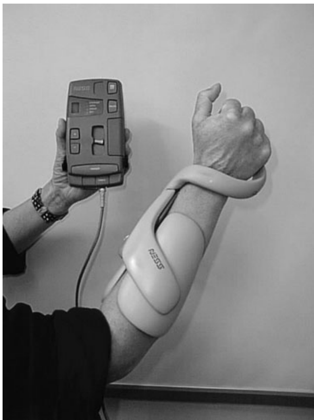
FIGURE 1. A hybrid brace-transcutaneous neuroprosthesis system that is worn on the hand and forearm. The exoskeleton positions the wrist in a functional position and the five transcutaneous electrodes built into the exoskeleton stimulates specific muscles to provide coordinated hand opening and closing. (NESS H200, courtesy of Bioness Inc., Santa Clarita, CA.)
