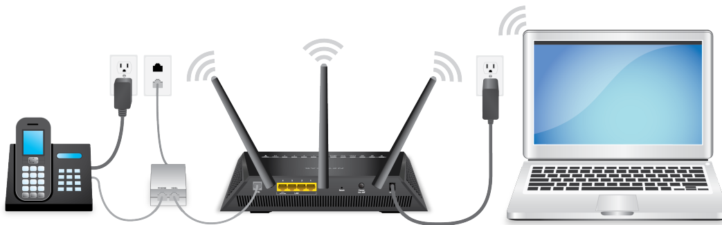
Figure 7. Modem router cabling for cable or fiber service
