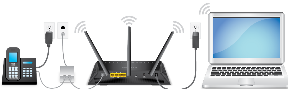
Figure 6. Modem router cabling for DSL service
