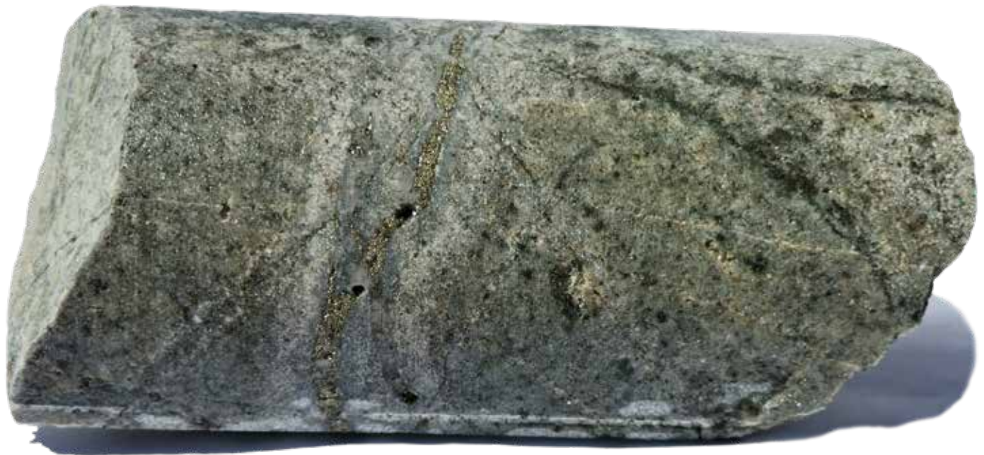
↗ Copper-bearing sulphide veins and disseminated copper sulphide mineralisation hosted within Intermineral Porphyry from the Hypogene Zone, Quellaveco Project.
