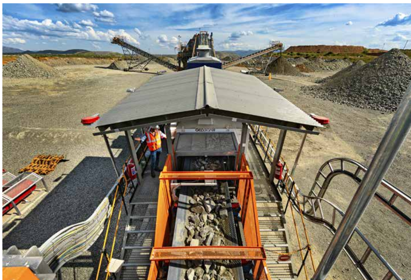
🔗 Bulk ore sorter, Mogalakwena mine.
