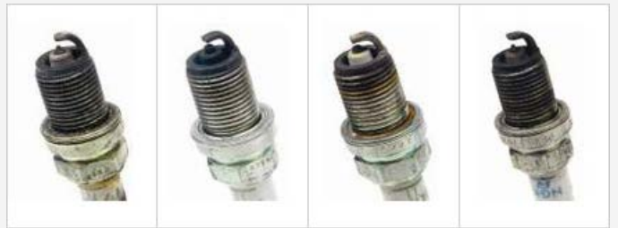
Worn Spark Plugs (Need to be replaced)
