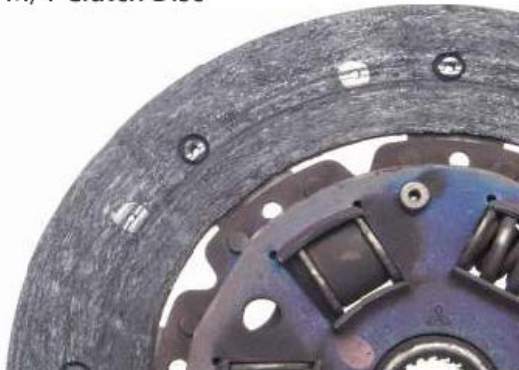
Worn out M/T Clutch Disc
