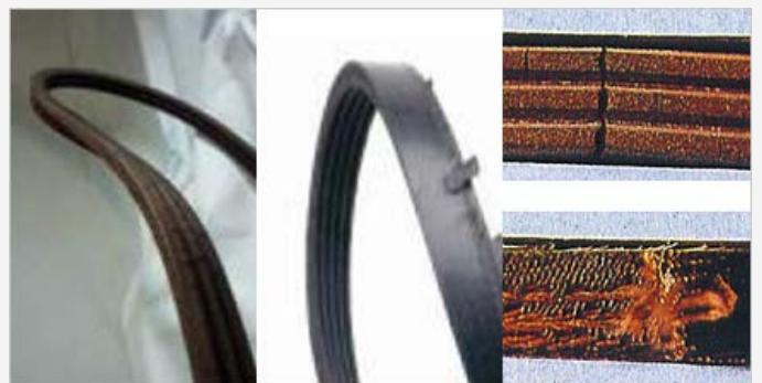
Used (Damaged: Need to be replaced)
