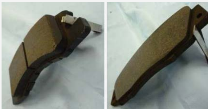
New (Enough Thickness)
