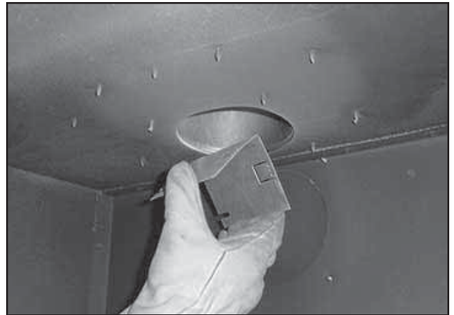
Figure 7.19 Placing the Baffle
