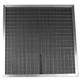
Electrostatic air filters utilize synthetic material which develops an electrostatic charge as friction is applied to the plastic fibers from the movement of air passing through it. The electrostatic charge that is developed as air passes through the filter increase the filter's attraction to particles such as pollen, molds and dust.
