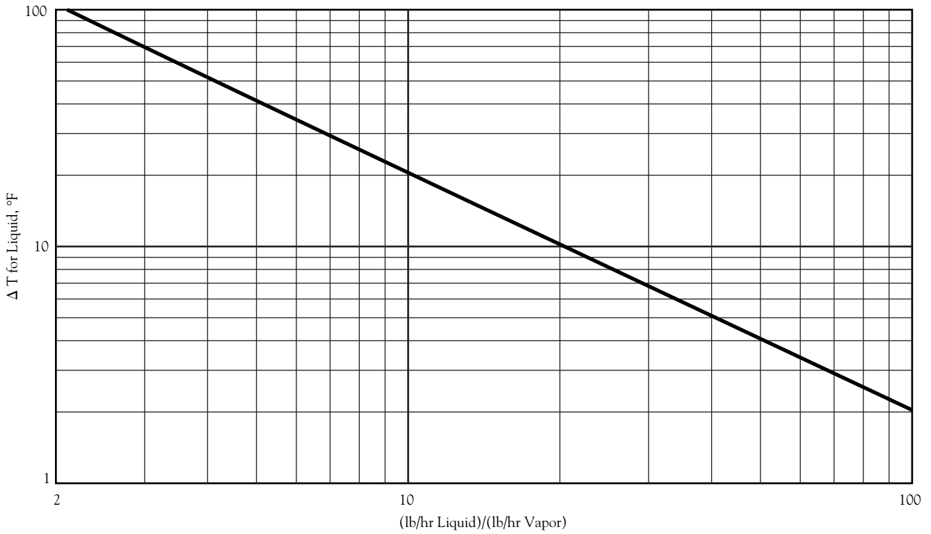
Figure 3—Comparison of Liquid vs. Vapor Mass Flow Rates for DOWTHERM A Fluid at Various Liquid \Delta t 's
