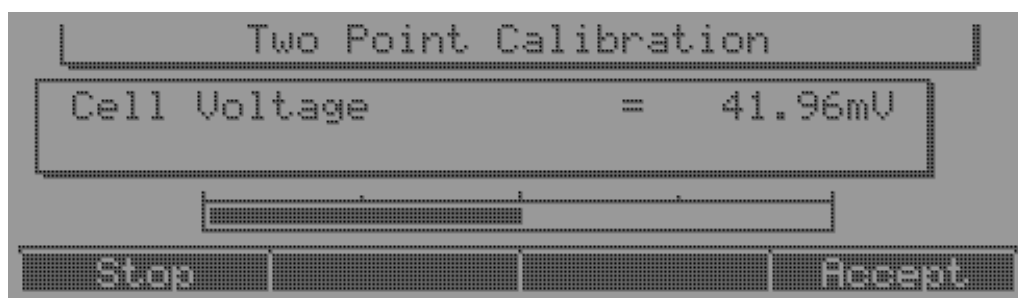
Figure 45 Display: O 2 two point calibration, 2.step (system without integrated pneumatic unit)
