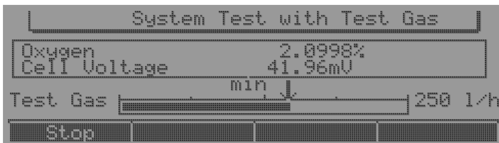
Figure 50 Display: System Test with test gas (system with pneumatic unit)
