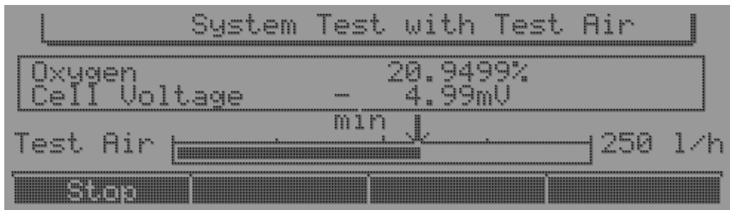
Figure 52 Display: System Test with test air (system with integrated pneumatic unit)
