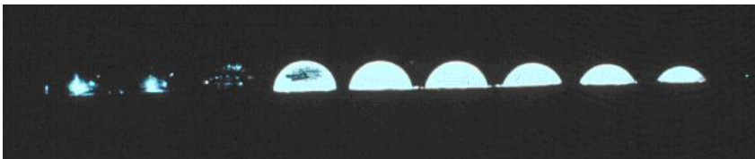
Figure 3-4. Effect of bead embedment depth on retroreflectivity.
