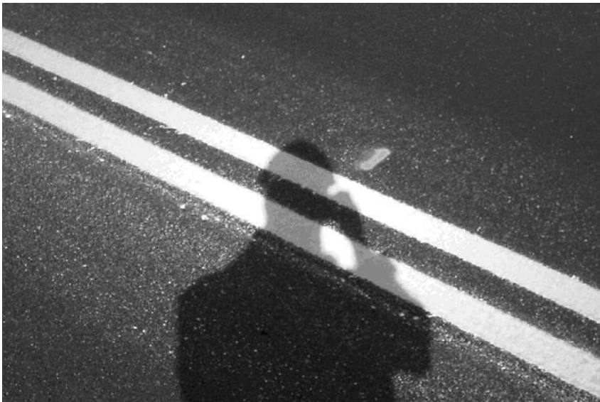
Figure 3-5. Sun-over-shoulder test from Test Method Tex-828-B.
