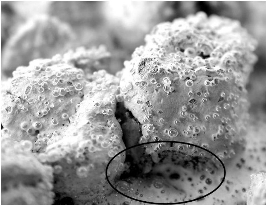
Figure 2-2. Beads falling between aggregates.
