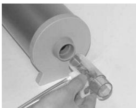
Figure 6.4. Proper connection of the flow meter to the calibrating pump.
