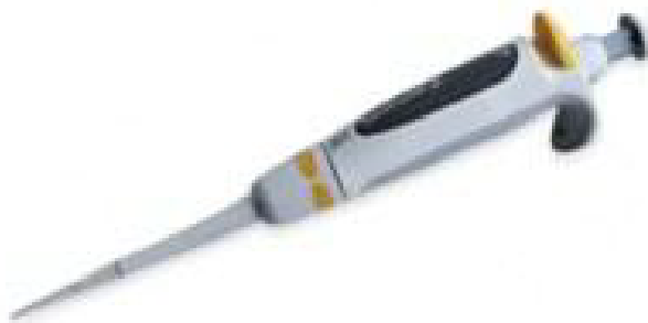
Fig. 4.3. Automated pipette with adjustable volume. Yellow colour indicates a volume between 2-20 \mu\text{l} , while grey coloured pipettes can be used between 100 to 1000 \mu\text{l} .
