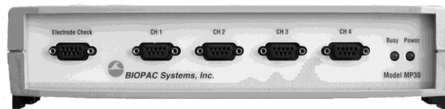
Figure 3.1. MP30 data acquisition unit. The device is connected to the computer by USB cable.
