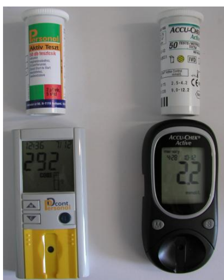
Figure 8.4. The D Cont personal and Accu check blood glucose meters and the corresponding test strips.
