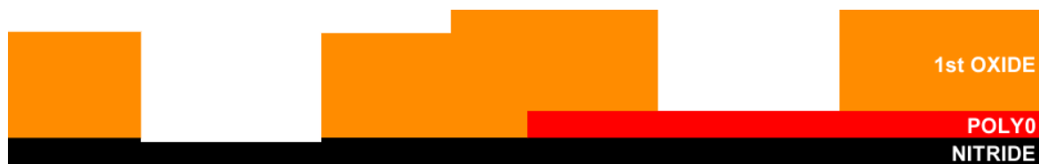
FIGURE 2.17. ANCHOR1 cuts down to Nitride and Poly 0. Note that the underlying Nitride has been partially etched (see fig. 1.1 for fill patterns).
