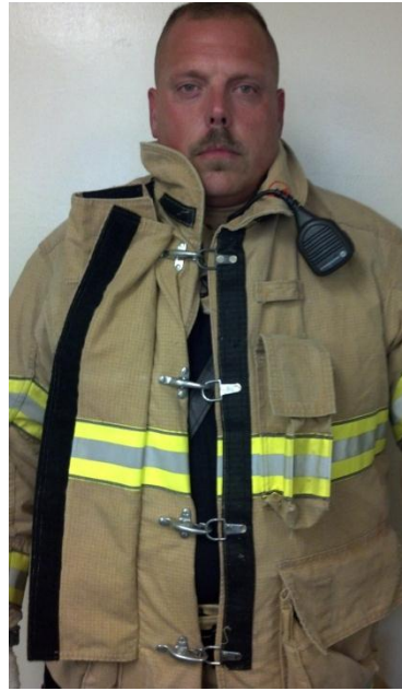
Figure 2 – Don coat, un-clip the RSM and place it to the side, clip all four buckles.
