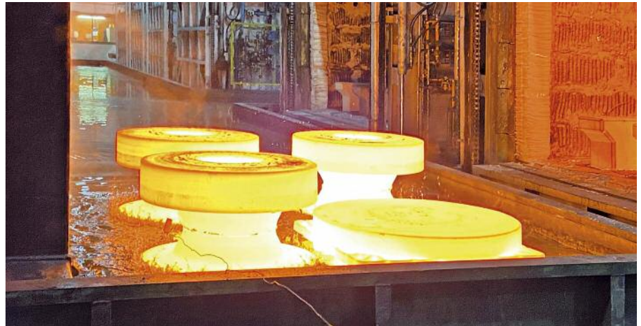
Water quenching of forged parts after they exit the solution annealing furnace. © Officine Ambrogio Melesi
