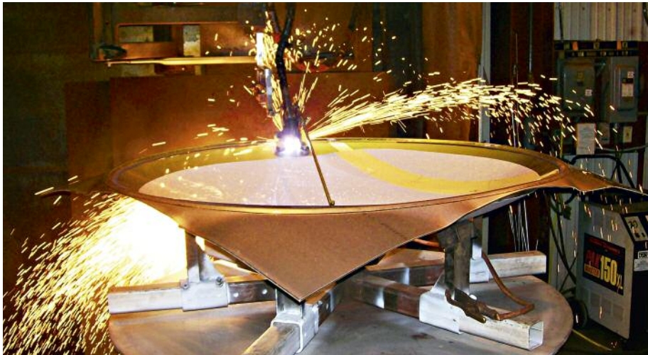
Plasma trimming of a GTA welded and hydro-formed austenitic stainless steel vessel head for sanitary applications. © DCI, Inc, St. Cloud, MN USA
