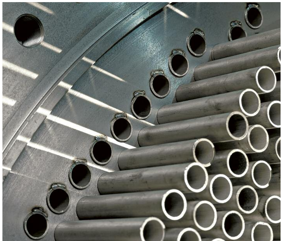
Heat exchanger tubesheet during fabrication. © Sandvik
