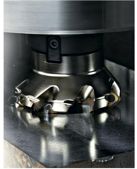
Face milling austenitic stainless steel with a carbide insert cutter. © Seco Tools
