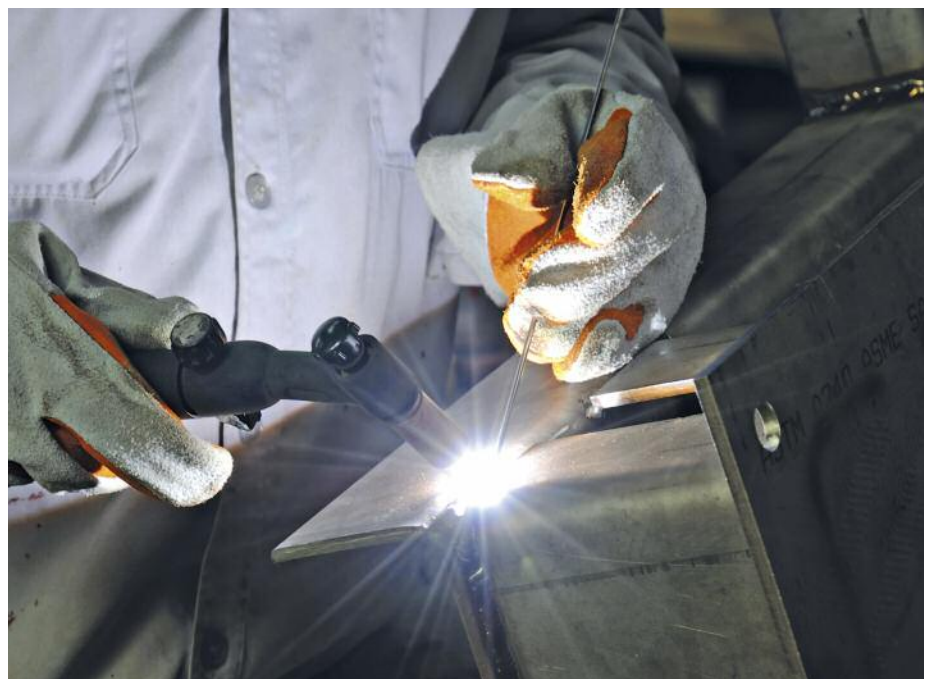
Manual GTA (TIG) welding. © iStock.com/Lekyum
