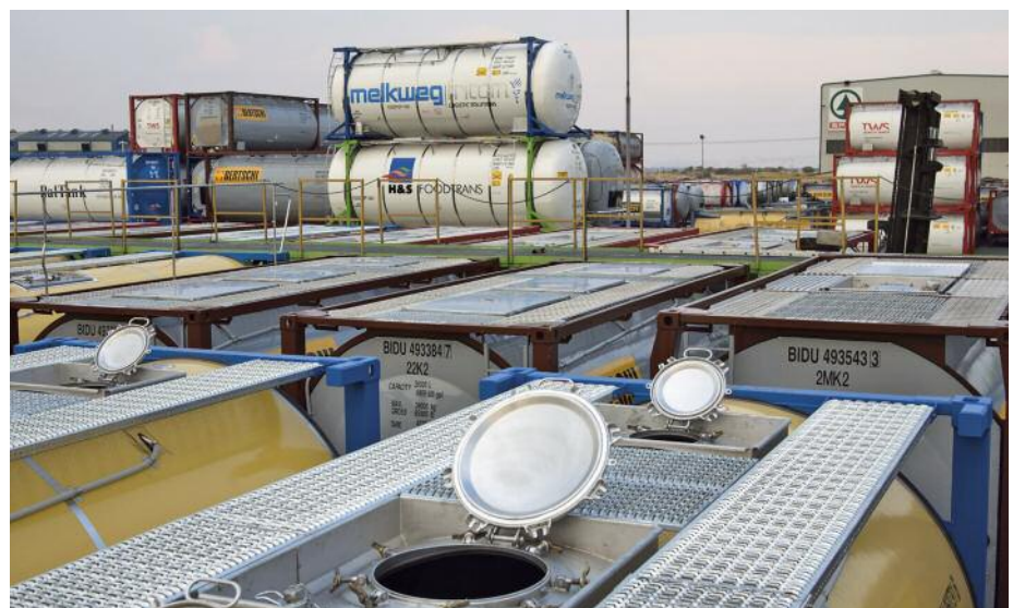
Intermodal tank containers are typically made of Type 316 stainless steel. They are cold formed into their cylindrical shape. © IMO A
