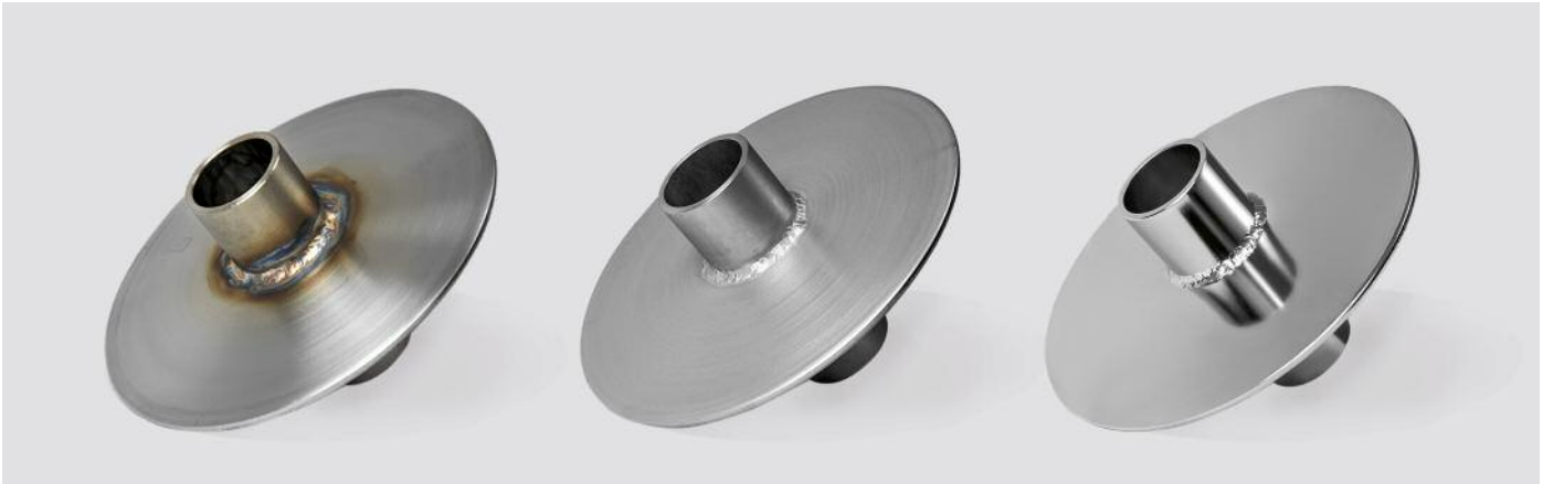
Post-fabrication cleanup of welded part: left: as welded, middle: pickled, right: electropolished. © Calamo AB
