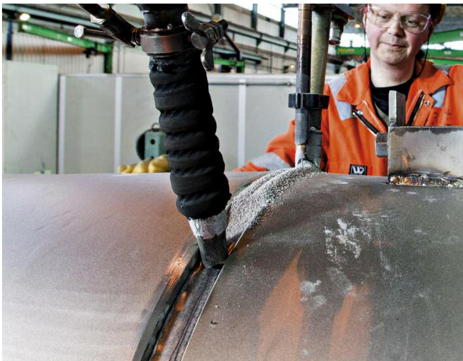
Submerged arc welding. © ESAB Welding & Cutting
