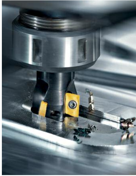
Side milling using carbide cutters. © Seco Tools
