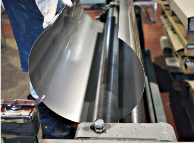
Three roll bending machine. © IMOA
