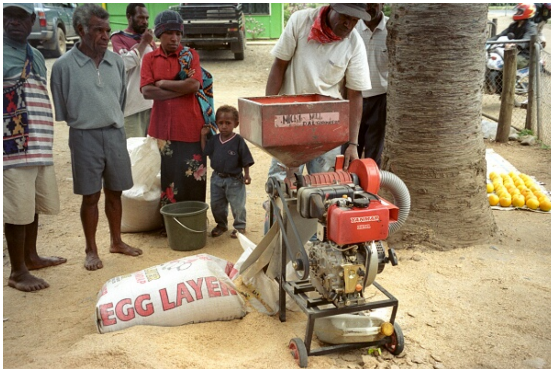
Rice bran milled in Goroka, PNG. The rice bran is ground to a fine powder during this process.
