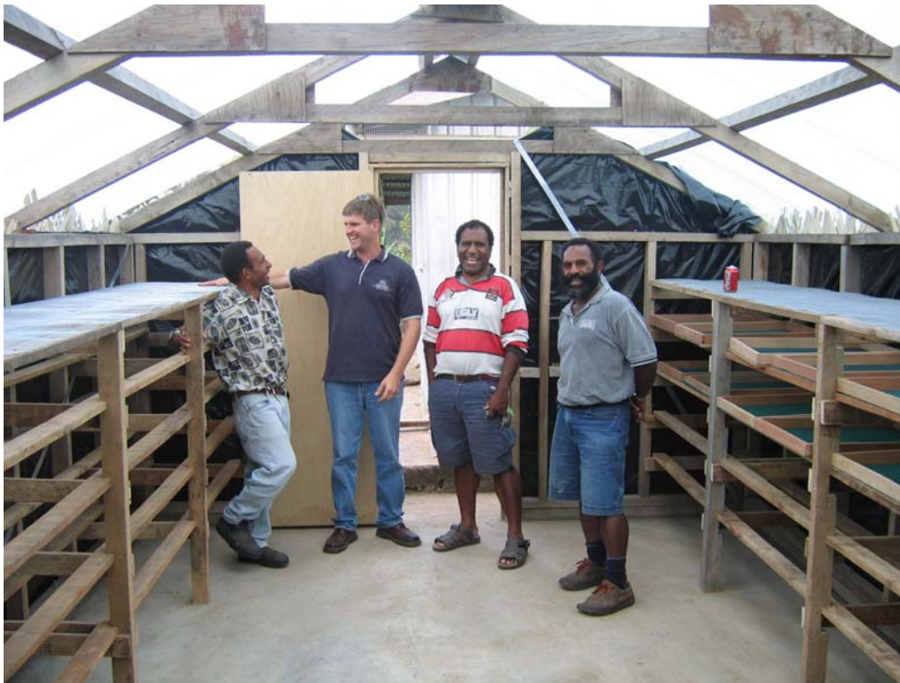
A simple solar dryer made from covering a timber frame with plastic. The air is drawn into the dryer through an open base, is heated by the sun in the dryer and exits through large gaps between the top of the walls and the roof.
