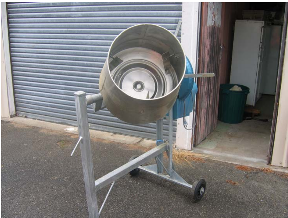
Ingredient mixer- a simple cement mixer is suitable to mix small batches of feed
