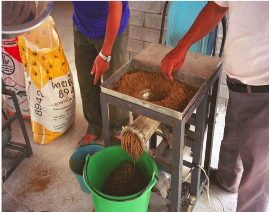
Pellet preparation using a pellet machine (mincer)
