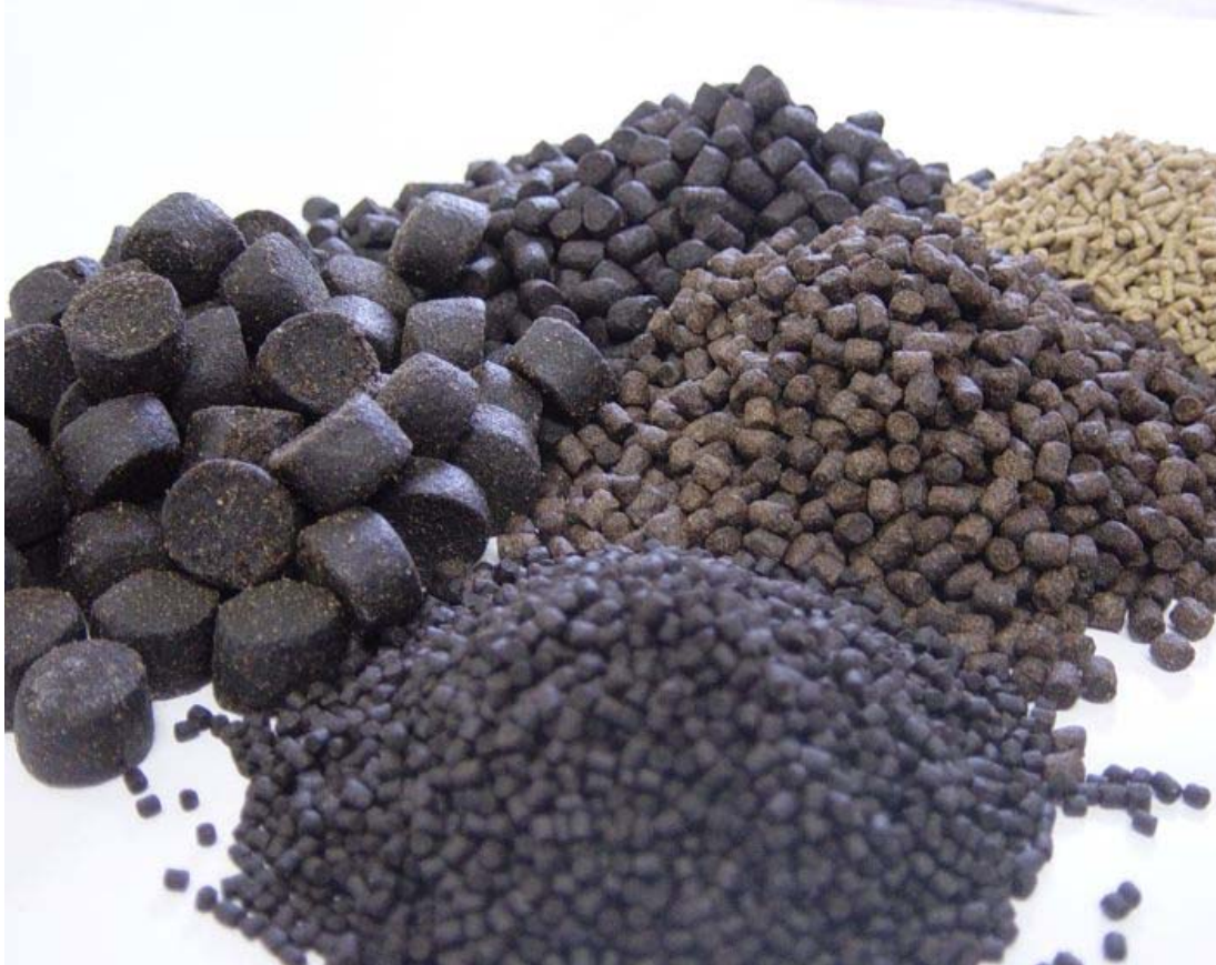
Pellets come in different sizes, shapes and colours. These are commercially produced extruded or steam pressed pellets
