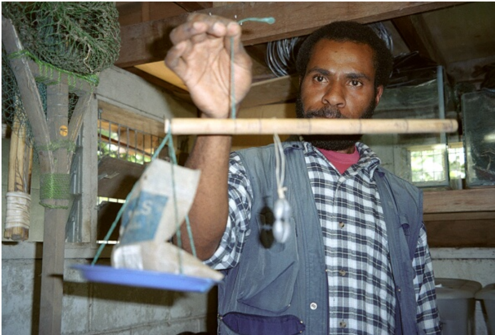
A simple balance is used to weigh ingredients at DAL Highlands station in Goroka, PNG
