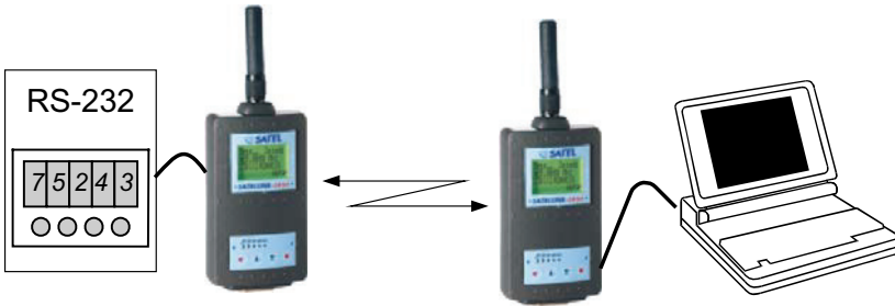
Figure 6.50. An example of measurement data wireless transmission (Satel 2005)
