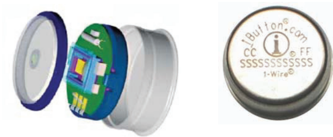
Figure 6.5 The temperature sensor iButton of the Dallas Semiconductor (Dallas Semiconductor 2005) (permission of Dallas Semiconductor)
