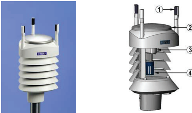
Figure 6.8. The Vaisala Weather Transmitter WXT510 (1 – wind transducers, 2 – precipitations sensor, 3 - pressure sensor, 4 – humidity and temperature sensors (Vaisala 2005) (permission of Vaisala Group)
