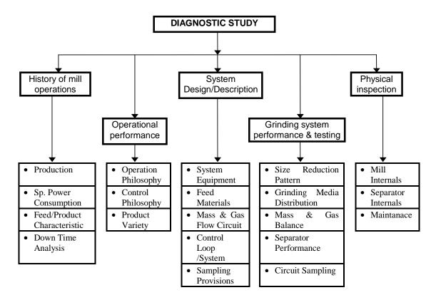
The mill performance is evaluated and recommendations are formulated based on the past history of the mill operations, inspections, process measurements, feed/product characteristics and grinding performance, in order to improve mill output and reduction in power consumptions in the ball mill system.
