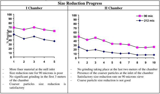
• . To assess he performance of the separator, circuit samples were collected and the results and observations on the same are given below:
