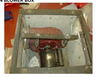
Photograph A2: The Inside of the Box Showing the Motor and the Blower Unit.
