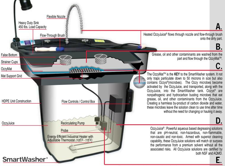
The 300 gph recirculating pump pulls the fluid from the tank sending it back through the nozzle and brush. OzzyJuice is ready to clean more dirty parts.
