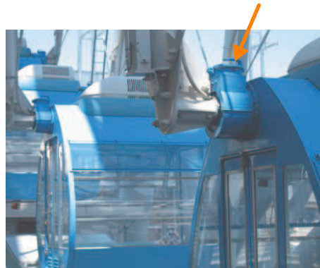
One-touch inspection doors installed on bearings of a Ferris wheel for inspection and lubrication
