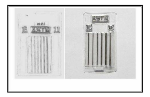
There are other IQI designs like the Hole/Plaque type and step wedge design.
