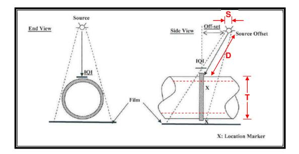
Exposure set-up for 2"  $\ensuremath{\ensuremath{\mathcal{O}}}$  Wall Thickness 5.6 mm.
