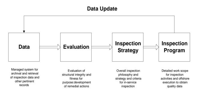
Figure 2: ISO procedure [2] for development of inspection plan
