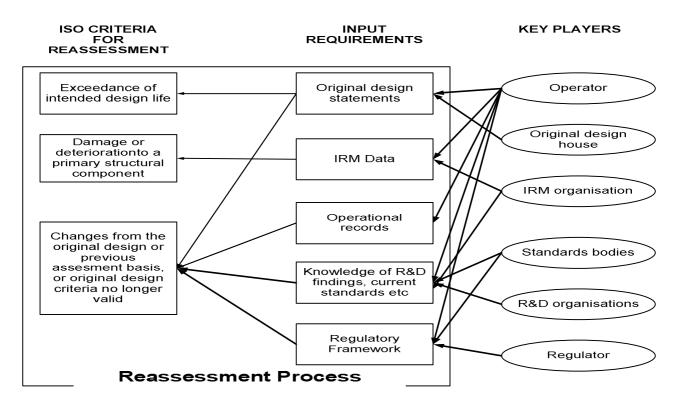
Figure 3: Reassessment process showing criteria, relevant input data requirements and key players
