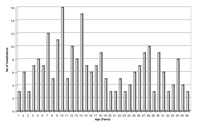
Figure 1: Histogram of fixed steel installations on UKCS by age
