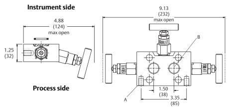
A. 3/8-16 UNC mounting holes (2) B. 1/2-14 NPT process connection (2)
