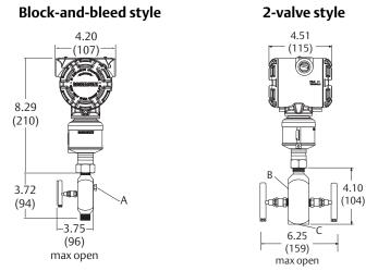
A. Bleed screw (unspecified dimension) - not C. <sup>1</sup>/2–14 NPT female NPT process connection (code BA) designed for accessory attachments.
