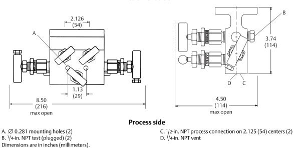
1. Manifold handle assembly may vary slightly from image shown. All valve handle assemblies provide the same function and meet all stated drawing dimensions.
