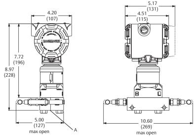
A. <sup>1</sup>/2–14 NPT on manifold for process connections, 2<sup>1</sup>/8-in. center-to-center, <sup>1</sup>/4–18 NPT for test/vent connection Dimensions are in inches (millimeters).
