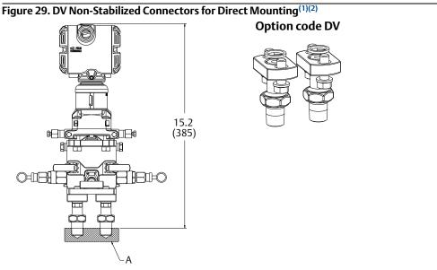
A. Cross section image is shown for dimensioning purposes only; it is not part of the transmitter assembly Dimensions are in inches (millimeters).
