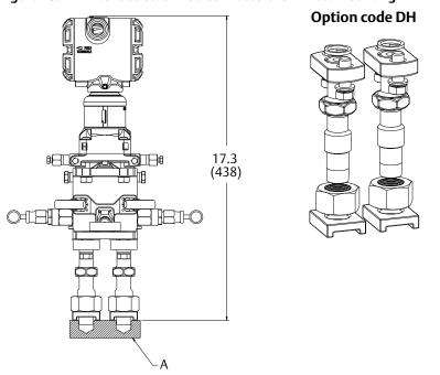
Figure 28. DH Extended Stabilized Connectors for Direct Mounting<sup>(1)(2)</sup>
