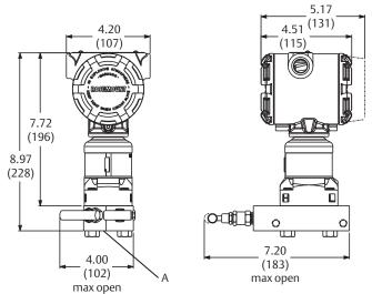
A.  $^{1}$ /2–14 NPT on manifold for process connection,  $^{1}$ /4–18 NPT for test/vent connection Dimensions are in inches (millimeters).
