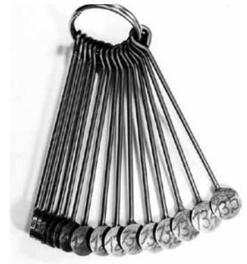
Fig. 49: Example of radius gauges (own production)
