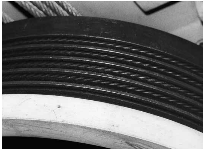
Fig. 51: Rope impressions in the grooves of a traction sheave
