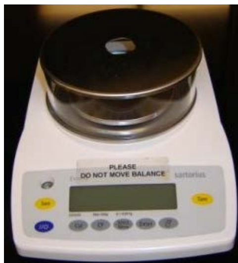
Figure 2-1. Sartorius Balance Model ED323S
